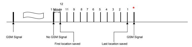
When the next real time tracking location (\*) needs to be sent back and the transmission is successful the WTGAT will try to send back the missed locations. Missed locations are sent back starting from the last saved location (1). One message (SMS or GPRS) will contain 4 locations.
