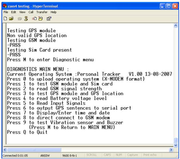
· With the WTGAT connected to the computer and in Diagnostic mode press 0 to begin the upload.
