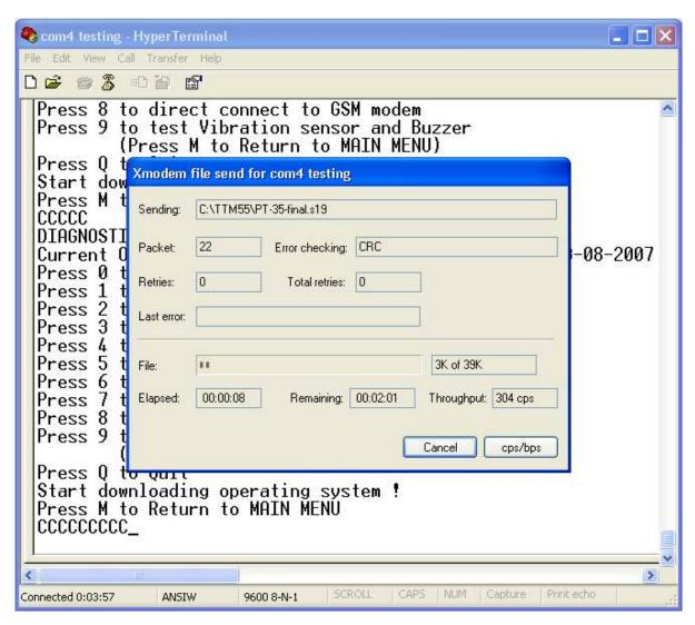
After upload the WTGAT unit will restart into the **Diagnostic Main Menu**. The Version and Date details of the new Operating System will be displayed.
