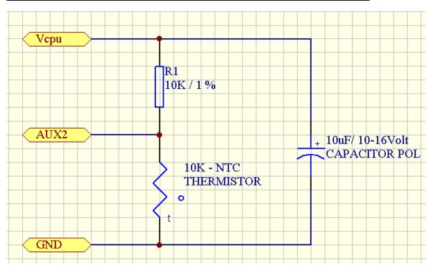
The AUX2 input voltage will change when the temperature changes. Most Thermistors are at normal resistance (in above example we use 10 K) at 25 degrees. So in our example that will be 10K. The input voltage to AUX2 will then be 1.27 Volt (ADC value will be 128 decimal or 80 hex).
